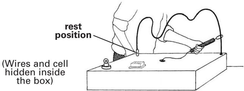
The metal ring and the thick wire both let electricity through.
